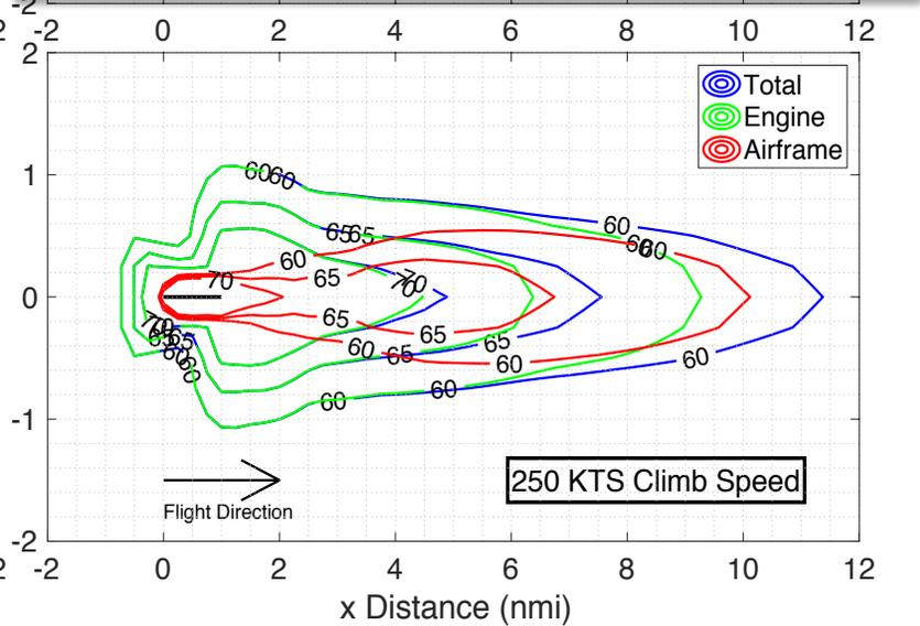
**Aerodynamic noise sensitive to “Wing Cleanliness” coefficient in ANOPP**
