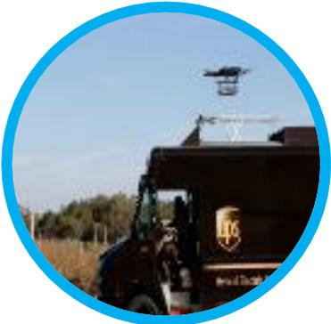
**UPS** UAS-integrated delivery van testing
