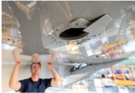
Noise-reducing vortex generators Image Source: Condor
