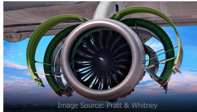
Ultra-high bypass geared turbofan engine
